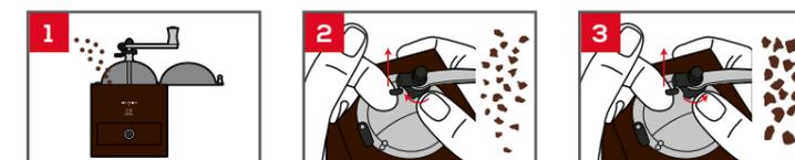
Réglage de la mouture / Adjustable grinding system
