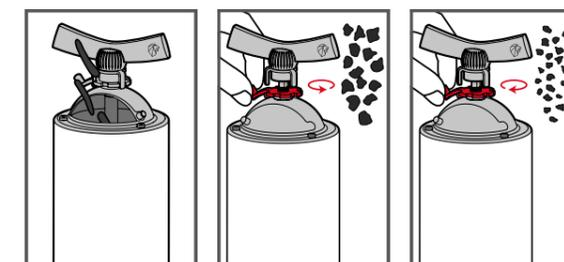
Réglage de la mouture / Adjustable grinding system
